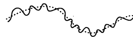
FIG. 2. Schematic representation of a fluctuating surface. The full line represents the surface in which fluctuations with wave number up to \Lambda are allowed. The dotted line represents the coarse-grained surface with maximum wave number of fluctuations less than \Lambda/b . Each element of area of the coarse-grained surface has greater mass than the original surface because of surface crumpling. The degree of crumpling can change locally causing the effective coarse-grained density to change and rendering the membrane compressible.
